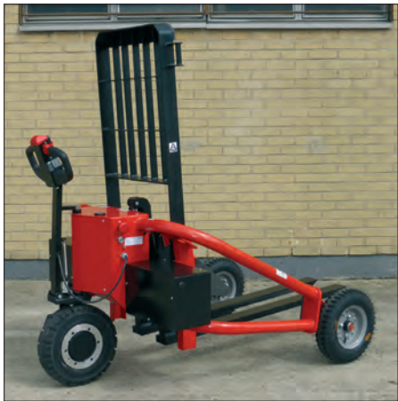
TNE with Tall Load Support and Load Strap
